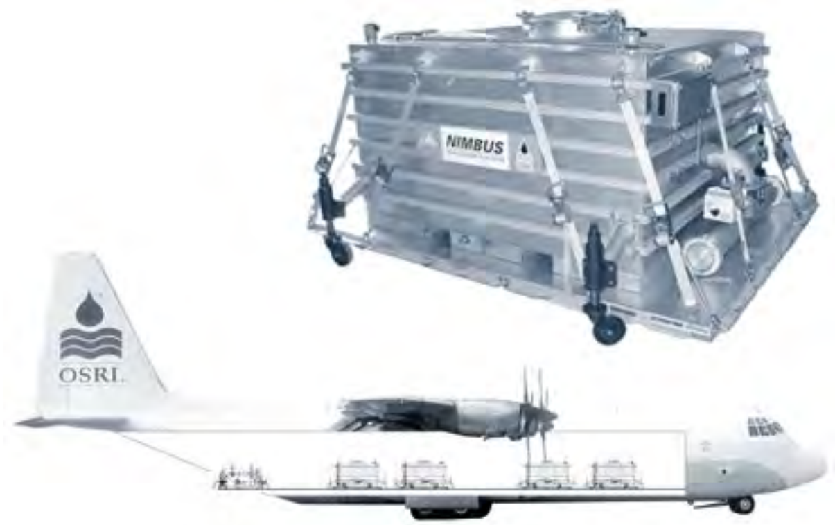
Figure 16. Lockheed L-382 Hercules aircraft with Nimbus spray system
