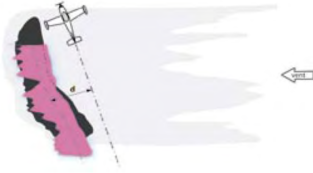
Figure 19. Spraying dispersant from a fixed-wing aircraft at an angle to the prevailing wind
