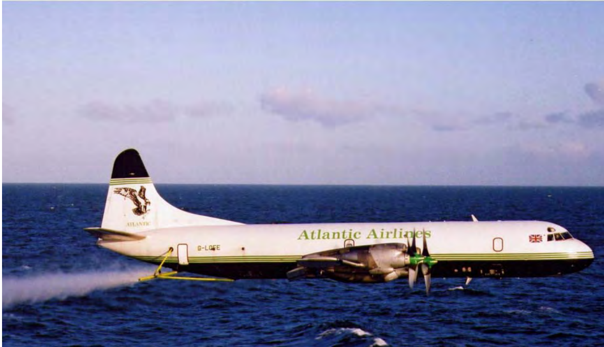
Figure 14. Lockheed Electra aircraft spraying dispersant
