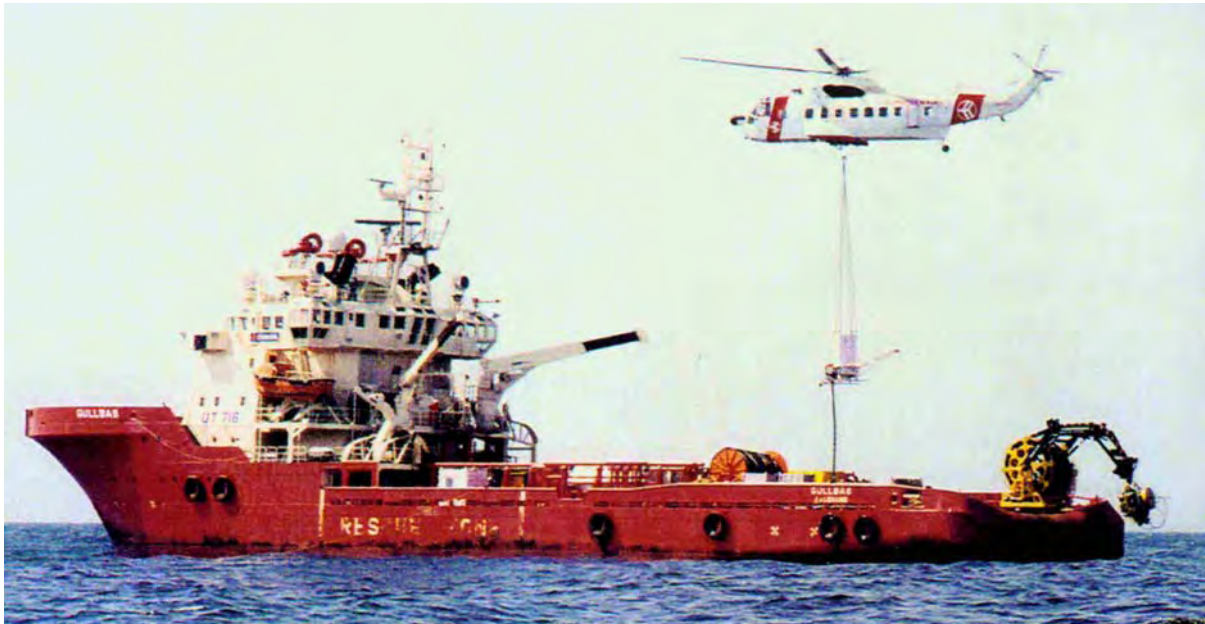
Figure 17. A Sikorski 61N helicopter reloading a RESPONSE 3000 dispersant spray bucket from dispersant stored onboard a support vessel
