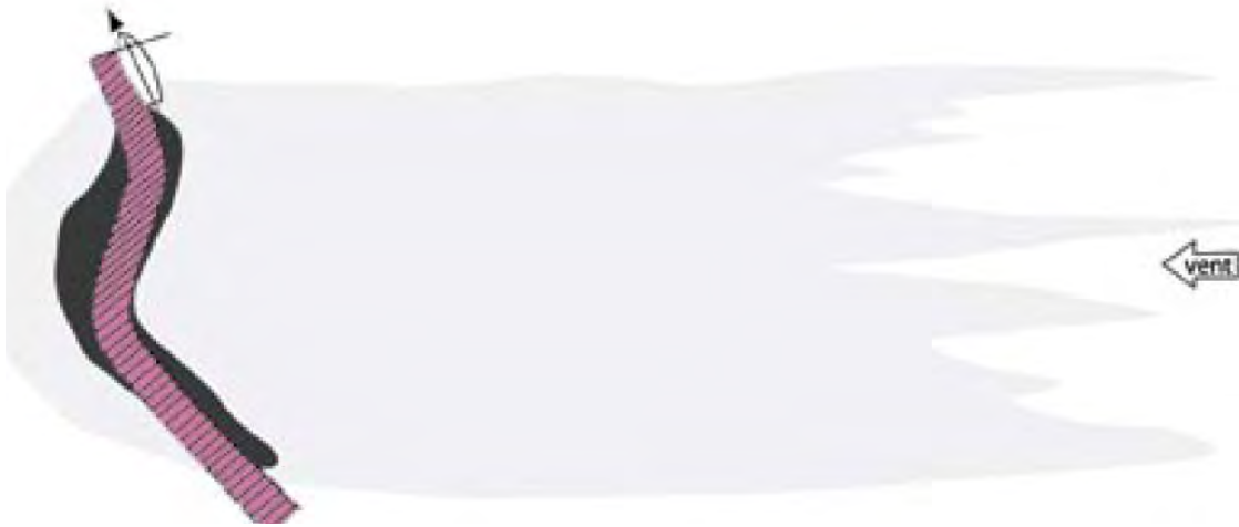
Figure 14. Spraying dispersant at an angle to the prevailing wind
