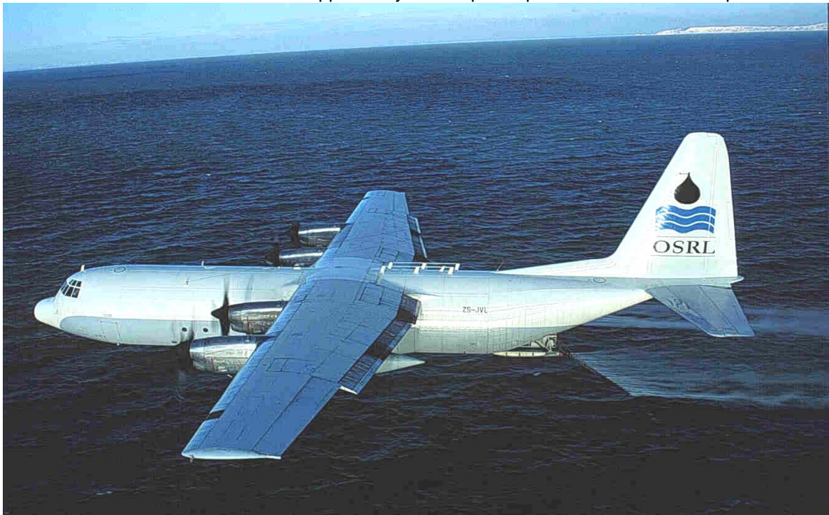
Figure 15. Lockheed L-382 Hercules aircraft with Airborne Dispersant Delivery System (ADDS Pack)
